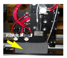
3. Pull the Z-axis brake release toward the front of the machine while pressing the Z-axis gantry downward into the foam.
