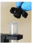
Figure 4-3: Replace Receiver Head
