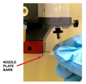
Figure 3-13: Attach Feed Tube to Nozzle Plate
