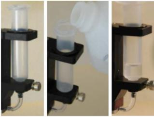
Figure 4-2: Install an Empty Syringe and Fill With Solvent
