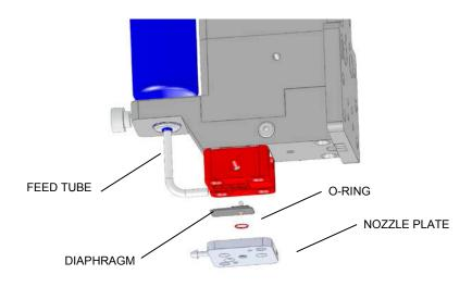
Figure 2-1: NCM7500 Nozzle Plate, O-ring, Diaphragm, and feed tube
