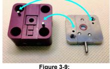
Alignment Pins on Heater Block
