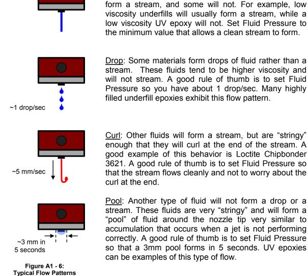
viscosity underfills will usually form a stream, while a low viscosity UV epoxy will not. Set Fluid Pressure to the minimum value that allows a clean stream to form.
