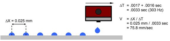
Figure A1 - 8: Calculating Robot Velocity for Drop Spacing = 0.025 mm, Refill Time = .0017 Sec and Dwell Time = .0016 sec
