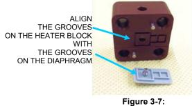
Figure 3-7: Align the Grooves
