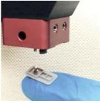
Figure 3-6: Press Diaphragm into Place
