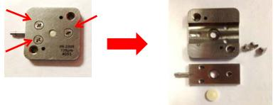
Figure 3-3: Disassemble the Nozzle Plate
