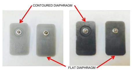
Figure A1 - 4: Contoured and Flat Diaphragms
