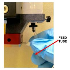
Figure 3-12: Attach Feed Tube and Insert Syringe
