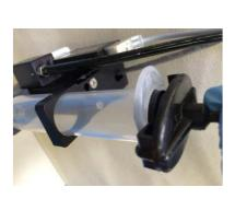
Figure 3-14: Install Receiver Head
