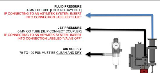
Figure 2-2: NCM7500 Pneumatic Connections
