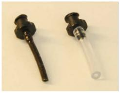
Figure A1 - 5: (I - r) Silicone and Tygon Feed Tubes
