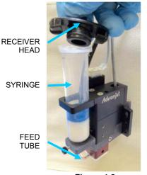
Figure 4-2: Disassemble and Remove Syringe
