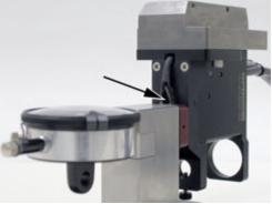
2. Gently pull the indicator pin away from the pump, cycle the pump several times, and verify the gap.
