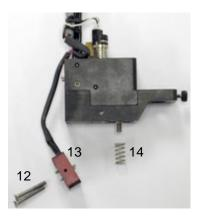
2. Remove and discard the compression spring (Item 14). For replacement parts, refer to NCM5000 Pump Maintenance Kit (22290043M).
