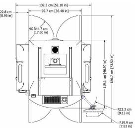
Left-to-Right direction of flow is standard; however Right-to-Left is configurable at time of order.
