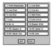
To open the Point Type window, press TYPE on the Point Edit window. For details about a specific type, refer to <a href="Programming Operations">Programming Operations</a> (pg 29)
