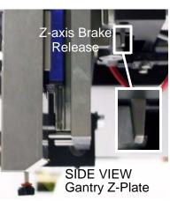
e. Depress the Indicator Point with a finger and then move the gantry to the right making sure the needle in Station #2 does not contact the Indicator Point.
