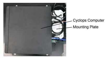
3. Slide the "side panel/Cyclops computer" assembly onto the computer tower and secure with the 3 bolts previously removed from side panel.
