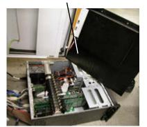
7. Remove the mounting plate and Cyclops computer from the side panel. Set the mounting plate aside. Dispose of the old Cyclops computer in a responsible manner.
