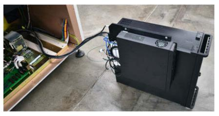
5. Disconnect all cables from the Cyclops computer. As needed, loosen any mounting plate clamps to allow the captured cable to be disconnected.
