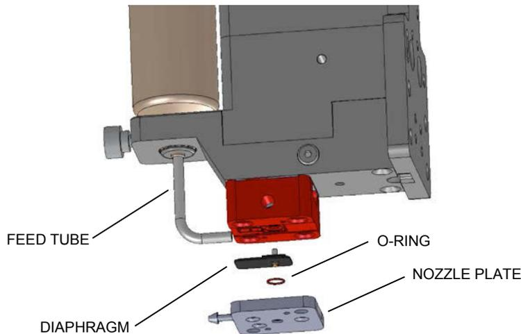
Figure 3-1: NCM7500 Heater Block, Diaphragm, O-ring and Nozzle Plate
