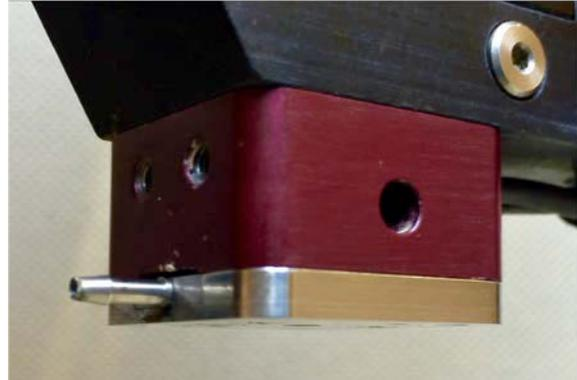
Figure 3-15: Check For Leaks at Weep Hole
