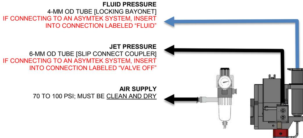
Figure 2-2: NCM7500 Pneumatic Connections
