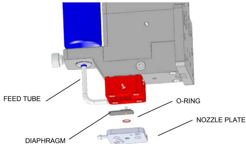
Figure 2-1: NCM7500 Nozzle Plate, O-ring, Diaphragm, and feed tube
