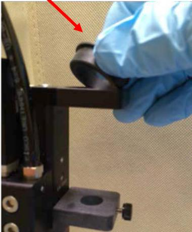
Figure 3-11: Insert Spacer Ring
