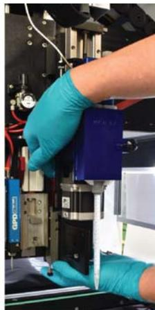
3 - Press Taper Lock lever down while seating valve.
