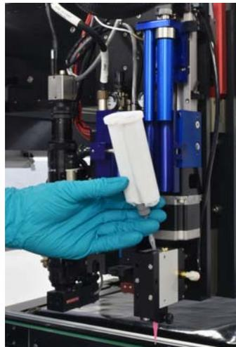
3. Install a Mixing Tube on a new material cartridge. Refer to [Installing Mixing Tube](#) (pg 3) for details.
