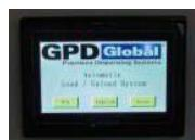
There is a color touch screen at the top of the machine. The operator can access it on the front of the machine. It is used to operate the machine and display machine status and information.
