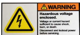
**WARNING:** High Voltage Electrical Risks - Do not touch cables or connectors before the machine has completely released all stored energy. The machine main power supply and several internal components are supplied with 230V AC. Direct contact with this voltage is very dangerous for human beings. Even if the machine is stopped by normal procedure or by pressing the E-stop button, some components and assemblies remained charged.
