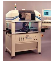
DS Micro II Heated dispense platform. Boards up to 15" x 9" (381 mm x 229 mm)
