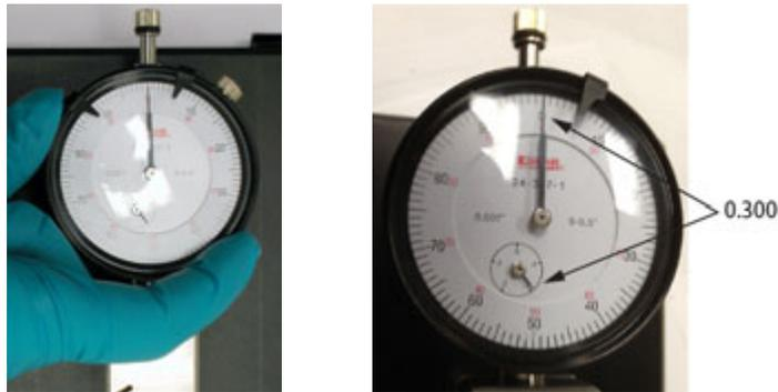
4. Gently pull the indicator pin and slide the gap tool tip protection tube back in place. Gently release the indicator pin.
