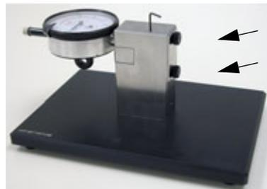
2. While pulling gently on the indicator pin, remove the gap tool tip protection tube. Carefully release the indicator pin against the zeroing plate.
