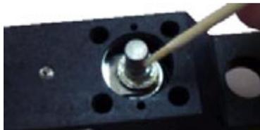
3. Locate the jet spring that was set aside and position it on the air cylinder tip.
