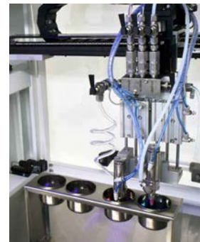
Valves at rest in Solvent Cups
